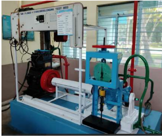
50 Diesel Engine Test Setup
