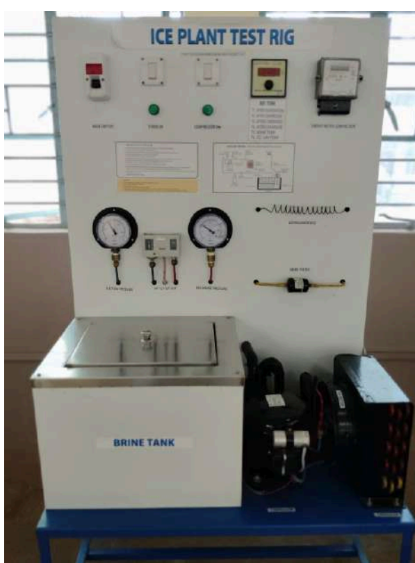
46 ICE plant test rig
